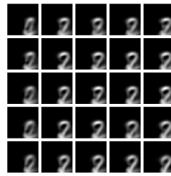
Fig. 5. Images restored using a shift invariant auto-encoder
