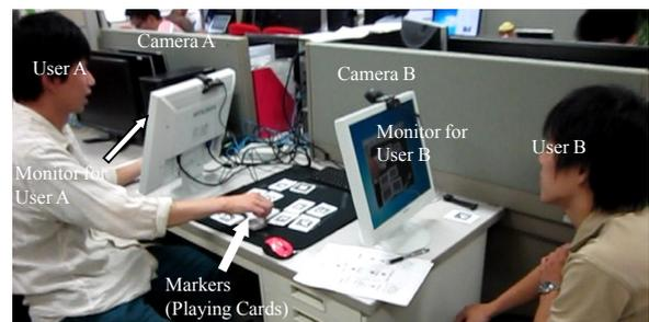
Fig. 1: An example of user-specific view with AR. Each user can see a different virtual world through his or her camera and monitor.
