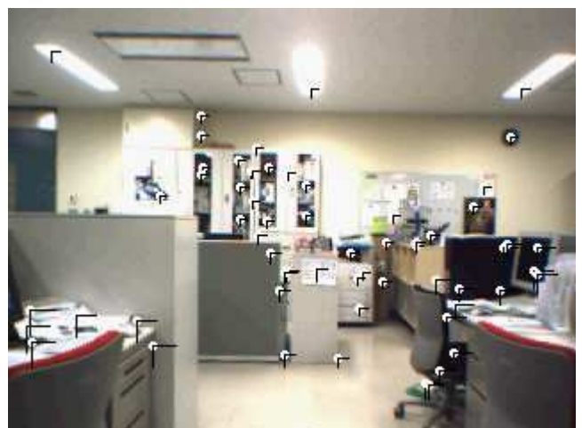
Figure 1 Trinocular correspondences: The white filled circles are the stable keypoints, the black lines from the stable keypoints are horizontal and vertical disparities.
