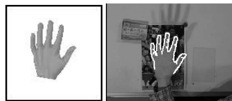
(c) Shape similar to input image (d) Edges of similar shape put on input image
